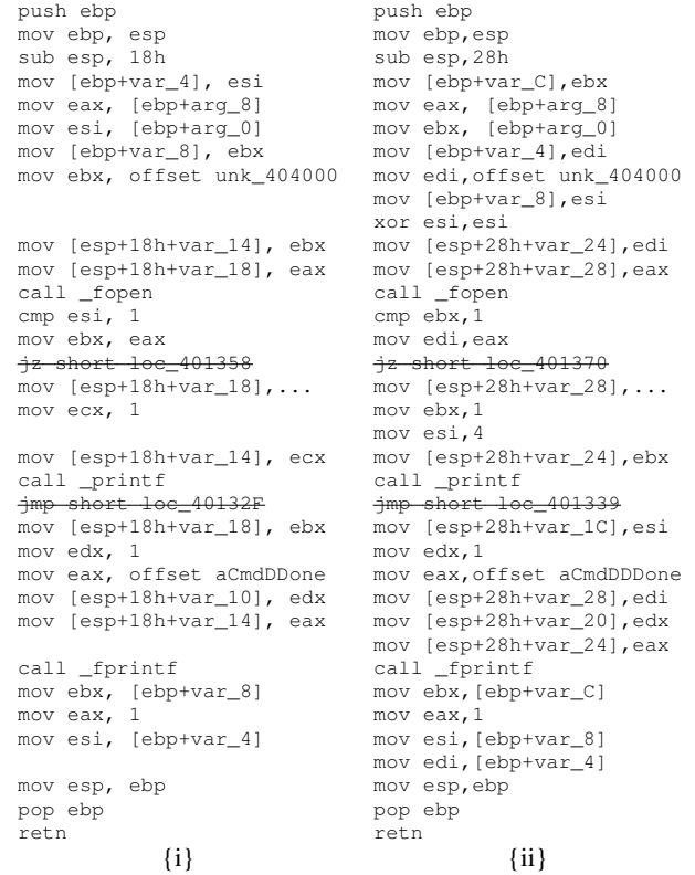
Figure 3. A pair of 3-tracelets: {i} based on the blocks (1,3,5) in Fig. 1(b), and {ii} on the blocks (1',3',5') in Fig. 2(b). Note that jump instructions are omitted from the tracelet, and that empty lines were added to the original tracelet to align similar instructions.
