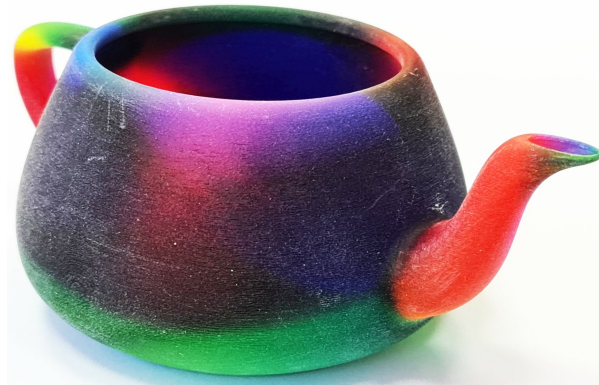
Figure 6: A 3D printed graded material V-rep Utah teapot model, from Figure 5, with fillets.
