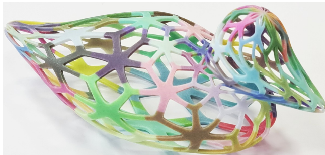
Figure 11: A shell lattice example. Semi-regular planar B-spline tiling is used to populate the domain of a duck B-spline trivariate shell, only to yield the presented result, after functional composition.
