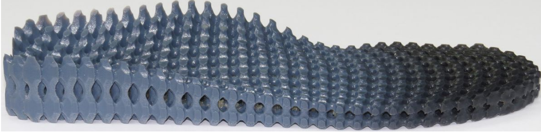
Figure 19: A 3D printed heterogeneous microstructure of a shoe sole. The front of the sole (in black) is flexible while the back size (in grey) is more rigid. Note the gradual change between the black and grey materials. Tiles from the family in Figure 14 (f).
