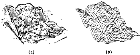
Fig. 4. (a) The terrain's 3D model. Size = 500 \times 770 mm. (b) The DTM constructed by using of a laser-based 3D-scanner. Grid spacing = 10mm
