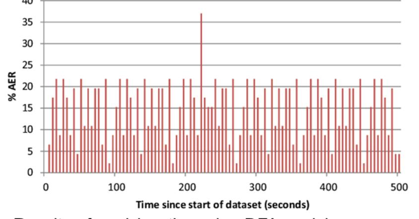
Results of applying the naive DFA model on a dataset of real Siemens S7-0x72 SCADA traffic
