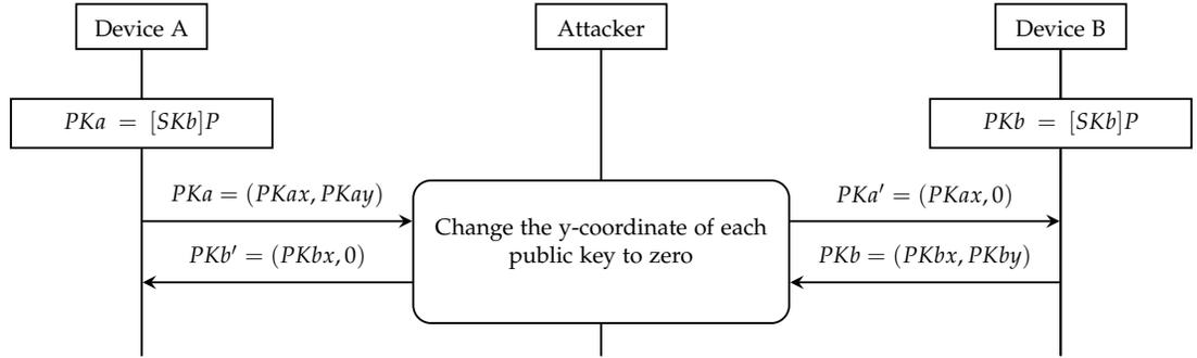
Figure 7: Semi-Passive MitM Attack – Passive Eavesdropping
