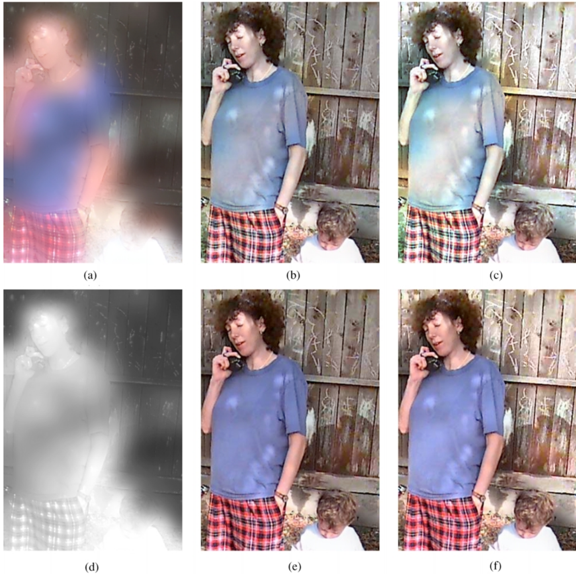
Figure 6. RGB retinex results: Illumination in (a) output with \gamma = 3 in (b), and \gamma = \infty (i.e. reflectance image) in (c); HSV retinex results: Illumination in (d) output with \gamma = 3 in (e), and \gamma = \infty (i.e. reflectance image) in (f).
