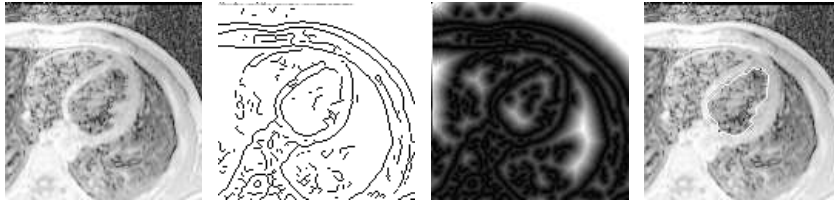
Fig. 4.2. MRI heart image, from left to right: Original image, edge image, distance map and Heart ventricle detection. The start point is on the lower left and the other one is the detected saddle.
