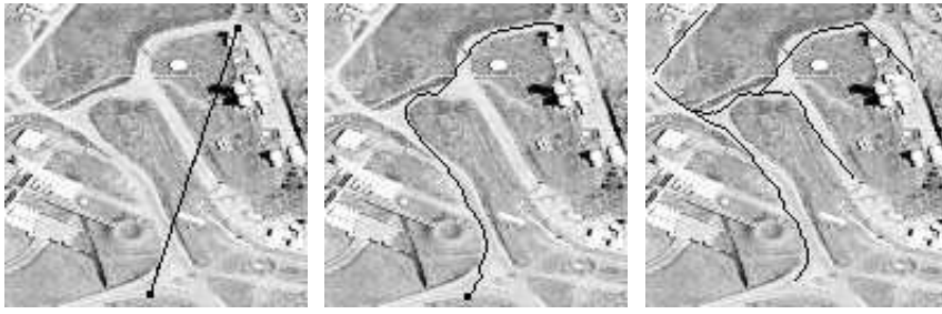
Fig. 4.1. The initial data is shown on the left. In the middle, our path of minimal action connecting the two black points as start and end points. On the right, many paths are obtained simultaneously connecting the start point on the upper left to 4 other points.
