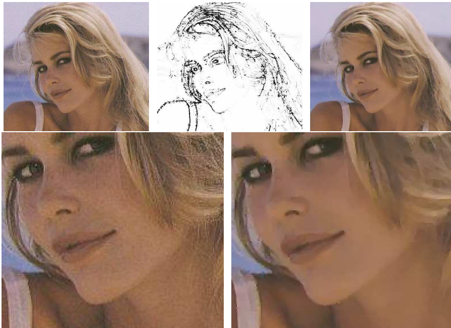
Fig. 2. Upper row, left to right: The original noisy image, followed by the final edge indicator function E , and the final image. At the bottom are zoom-in frames of a square section cropped from the initial and final images.
