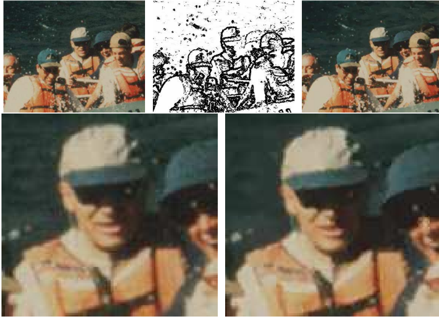
Fig. 4. The original noisy image is on the left, followed by the edge indicator field E , and the final result. Bottom line shows a zoom in on the original noisy on the left and filtered image.
