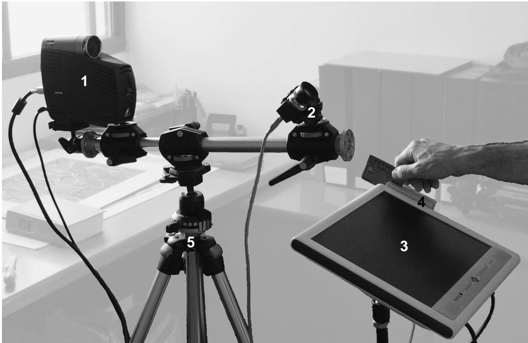
Figure 8: The 3DFACE prototype system and its main components: DLP projector (1), digital camera (2), monitor (3), magnetic card reader (4), mounting (5) .
