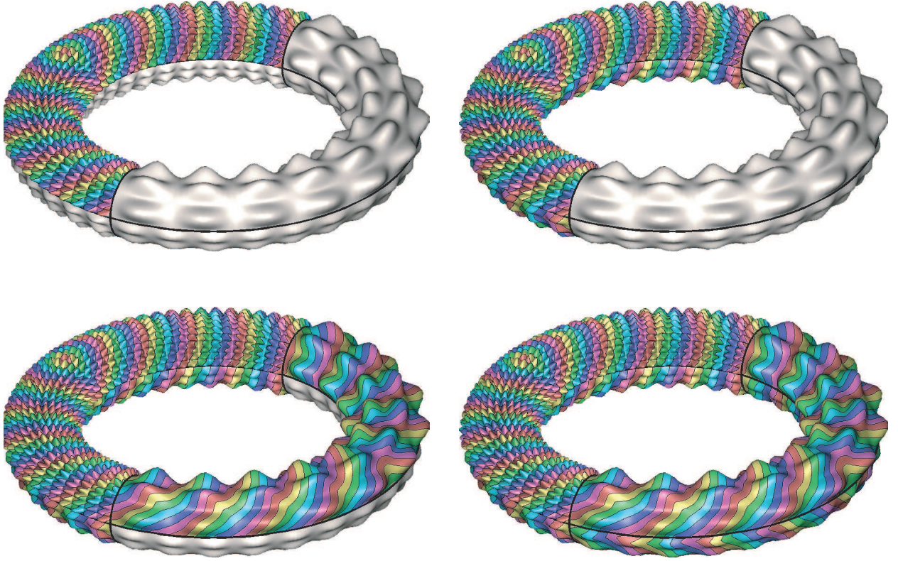
Fig. 13. Left-to-right bottom-down: the progress of the multi-chart fast marching algorithm on the bumped torus geometry image from Figure 12. First, the distance map from the source point is computed on the upper left chart. The distance values on the boundaries are extrapolated onto the neighboring charts, in which the distance maps are computed subsequently in the order of the minimum distance value on the boundary. Color map depicts the level sets of the distance map. In this example, a single pass of the algorithm gives an accurate distance map.
