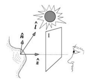
Figure 1. According to the simplest shading rule  $I=\langle \hat{l},\hat{n}\rangle$ , where  $\hat{n}$  is the surface normal.
