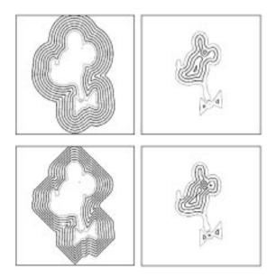
Figure 5. A dilation and erosion operations with diamond and circle structuring elements of different scales.
