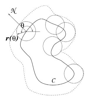
Figure 4. Dilation operation with a circle structuring element. In this case, since  $\sup_{\theta} \langle r(\theta), \vec{\mathcal{N}} \rangle = 1$  the evolution rule is simply  $C_t = \vec{\mathcal{N}}$  (i.e., the offsetting/prairie-fire problem).
