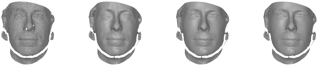
Figure 9: Left-to-right: raw range-scanned data triangulated into a surface, moving-least-squares results using PCL [RC11], and the results of phase I and II of the proposed algorithm. Note the delicate structures such as the eye and lip areas, and the relative smoothness of the forehead.
