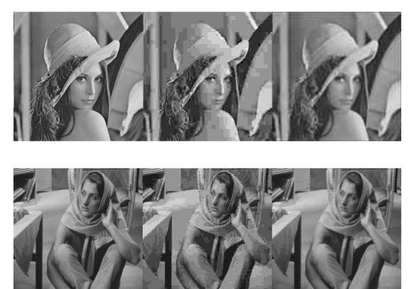
Fig. 2. Original image (on the left), JPEG compressed-decompressed image (middle), and down-sampled-JPEG compressed-decompressed and up sampled image (right). The down-sampling factor was 0.5. The compressed  $256 \times 256$  "Lena" image in both cases used 0.25 bpp inducing MSEs of 219.5 and 193.12, respectively. The compressed  $512 \times 512$  "Barbara" image in both cases used 0.21 bpp inducing MSEs of 256.04 and 248.42, respectively.
