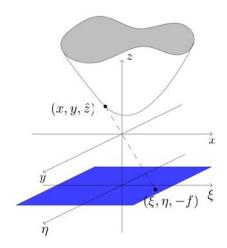
**Fig. 1.** Schematic representation of a surface taken under perspective view. The point of the real surface  $(x, y, \hat{z})$  is projected in the perspective domain in the point  $(\xi, \eta)$  of the focal plane (in blue), parallel to the optical one (xy-plane) at a focal distance f.
