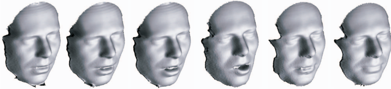
Fig. 1. Example of deformations of nonrigid surfaces: a video sequence of one author's face, acquired using a real-time 3D scanner. Facial expressions can be modeled as near isometries of the reference facial surface ("neutral expression").
