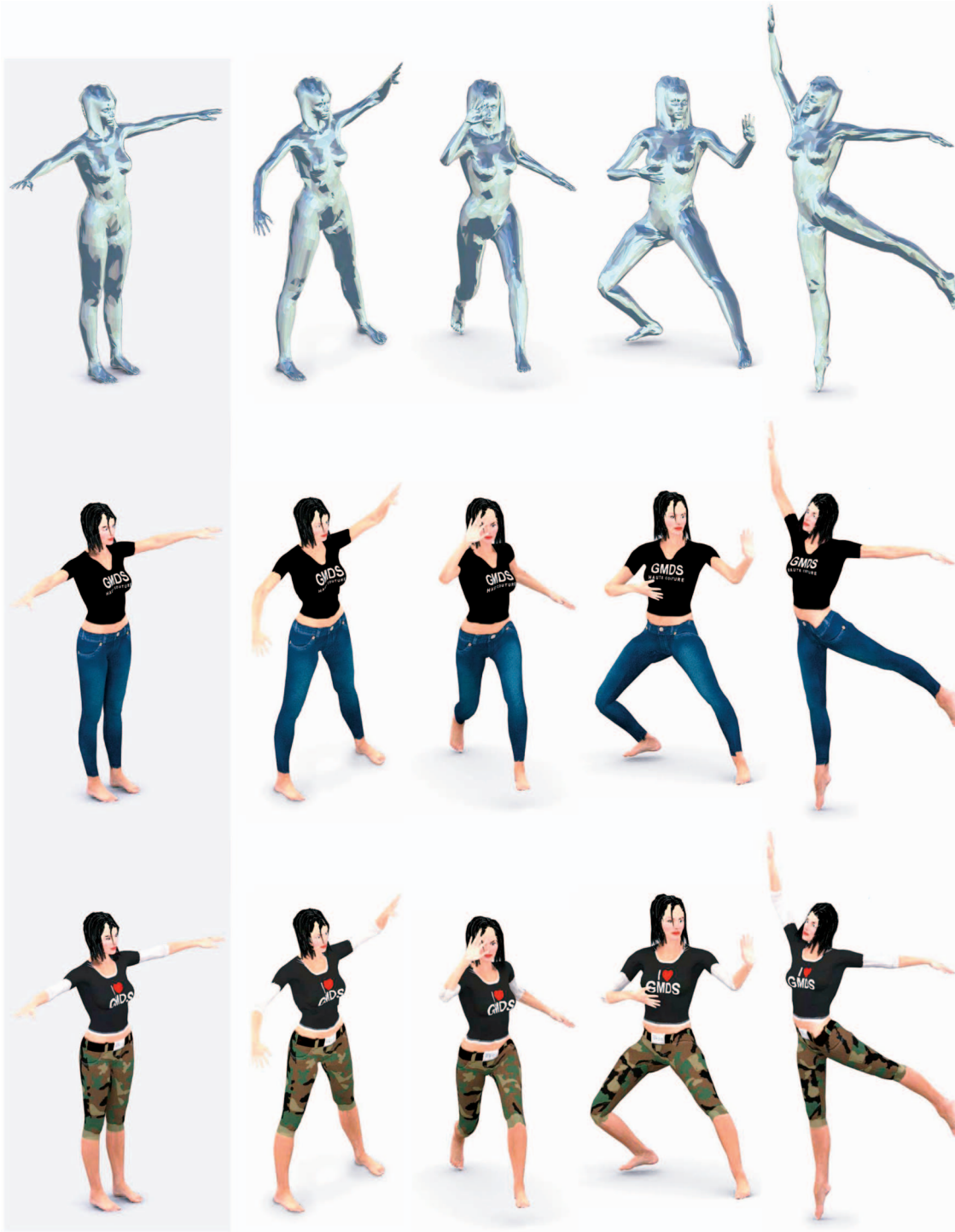
Fig. 5. Virtual body painting experiment. The texture is transferred from a reference pose of the human body (left column, outlined in gray) to its different poses. The correspondence between the objects is established by embedding 200 points on the reference object into its poses using the GMDS algorithm.
