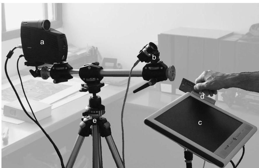
Figure 9. The 3DFACE prototype system and its main components: DLP projector (a), digital camera (b), monitor (c), magnetic card reader (d), mounting (e) .
