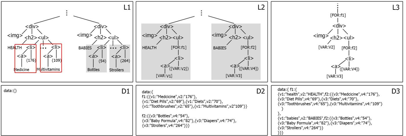
Figure 6: Example steps of the separation algorithm.
