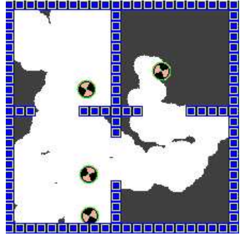
Figure 2: Four PC robots working together. A fellow robot is considered as an obstacle, hence no collisions should occur according to the PC rule.
