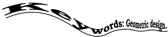
Figure 7. Layout of the string along the base curve without arc-length reparameterization. Compare with Figure 4.
