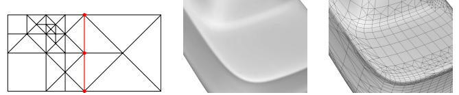
Figure 7: Seamless rendering of an adaptively subdivided mesh requires a valid mesh structure – no T-junctions.
