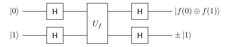
We can determine whether or not f(0) = f(1) with a single call on a circuit that computes function f.
