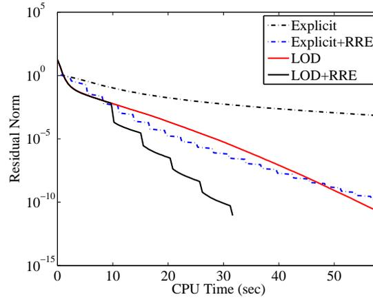
**Fig. 4.** Graph of the residuals (LOD, explicit+RRE and LOD+RRE) versus CPU times. Parameters:  $\Delta t = 0.05$  for the explicit scheme,  $\Delta t = 2.5$  for LOD,  $\lambda = 0.5$ ,  $\beta = \sqrt{500} \approx 22.36$ .
