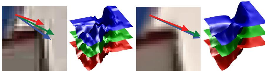
**Fig. 2.** The different image channels of an image patch taken from the images in Figure 1. Left to right: An image patch before denoising, its different color channels, the denoised image, and the denoised color channels. The color arrows indicate the direction of the gradient in the various color channels.
