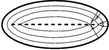
**FIG. 4.** One way to compute the distance from the (bold) ellipse is to propagate the curve along its normal with constant velocity. The set of curvature singularities (shocks) of the propagating wave is one possible way to define the symmetry axis of the shape (dashed bold line).
