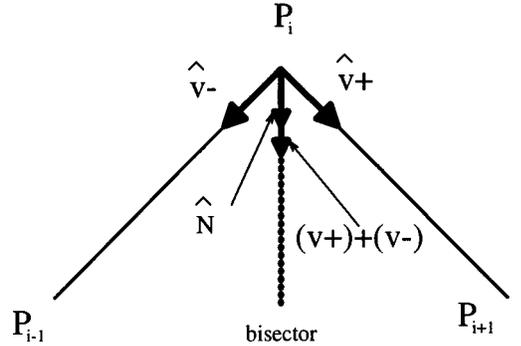
**FIG. 8.** The vectors  $\hat{v}_-$  and  $\hat{v}_+$  are defined by the vertices  $P_{i-1}$ ,  $P_i$ , and  $P_{i+1}$ . The dashed line indicates the bisector of  $P_i$  which coincides with the direction of the vector  $\hat{v}_- + \hat{v}_+$ .
