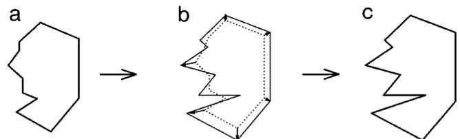
**FIG. 7.** Polygon exaggeration. For each vertex of the initial polygon (a), the normal  $\hat{N}_i^{(n)}$  and curvature  $\kappa_i^{(n)}$  are calculated. Then, (b) each vertex is moved in the direction of  $\hat{N}_i^{(n)}$  by a step proportional to  $\kappa_i^{(n)}$  thus creating a caricature effect (c).
