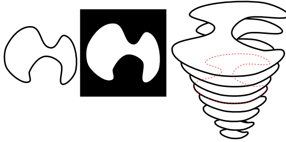
FIGURE 3. Left: A given planar curve. Middle: An implicit representation of the curve as a threshold set of a gray level image. Right: An implicit representation of the curve as a level set of a smooth function displayed by its level set contours.
