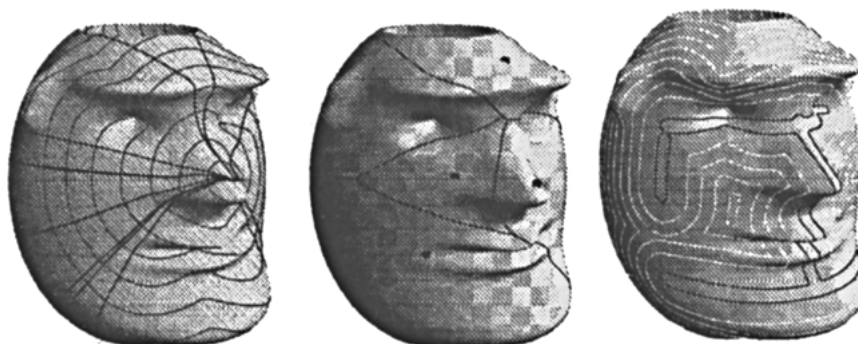
Figure 5. Fast marching on triangulated surfaces: Minimal geodesics, Voronoi diagram, and geodesic offsets.
