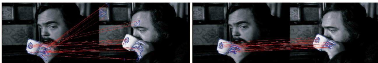
Fig. 5. Feature matching in two frames of a video using classical MSER  $\Psi_1$  (left) and our stability criterion  $\Psi_3$  (right).
