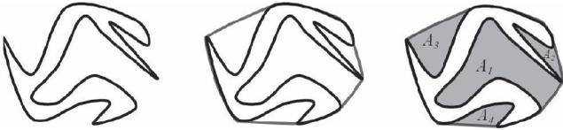
Fig. 2. Left to right: The shape's boundary contour, its convex hull, and the areas formed between the convex hull and the shape. The largest area,  $A_1$  in this case, defines the bitangent that is used for normalization (canonization) of the shape or for fixing its orientation.
