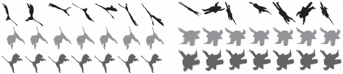
Fig. 1. First row: Random affine transformations of the silhouettes of the Puma logo (left) and a boy (right). Second row: Normalized shapes with second-order moments. Third row: Results of alternative method proposed by Cao et al.
