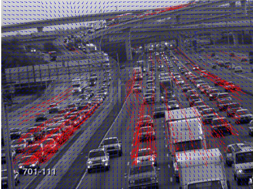
**Fig. 2.** Regularization of principal motion directions. The red arrows demonstrate measurements of motion cues based on a normalized cross-correlation tracker. Blue arrows demonstrate the regularized directions fields.
