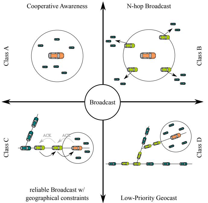
Fig. 1. Our vision of VANET broadcast classes: Class A for medium priority CAMs; Class B to forward highest priority events within  $N$  hops; Class C for high priority reliable broadcasting with geographical constraints; and Class D for low priority geocasting.
