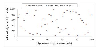
Figure 11: The acknowledgment field number of ACKs considered by the LB as ACK3 (representing legitimate connections) and of ACK3 packets sent by the client throughout the system running time
