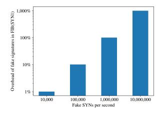
Figure 6: The overhead of recording fake signatures by FIB(SYN1) in Procedure-2b, as a function of  $r_{fake}$
