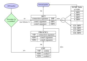
Figure 4: The flow of ACK packets coming from the clients in Procedure-2a
