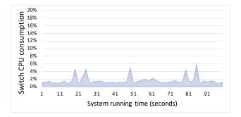
Figure 10: The switch's CPU consumption over the system running time
