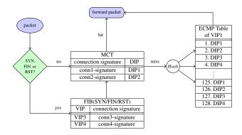
Figure 1: Packet flow for a specific VIP (VIP1) in Prism
