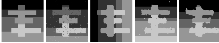
Fig. 4. The dependency of the query count on the error type. The five segmentations above differ in the source of the errors. The leftmost image gets all its errors from splits and merges, while as we move to the right, the influence of attached errors and noise is stronger. The number of queries required for these hypotheses are 51, 623, 593, 914 and 1368. (Corresponding quality values ( Q_T ) are 0.987, 0.87, 0.84, 0.76, and 0.64.) The corresponding difference measures are 10601, 10243, 10001, 9946 and 9916. Note that even though the difference measure stays the same or even decreases, the number of queries significantly increases.
