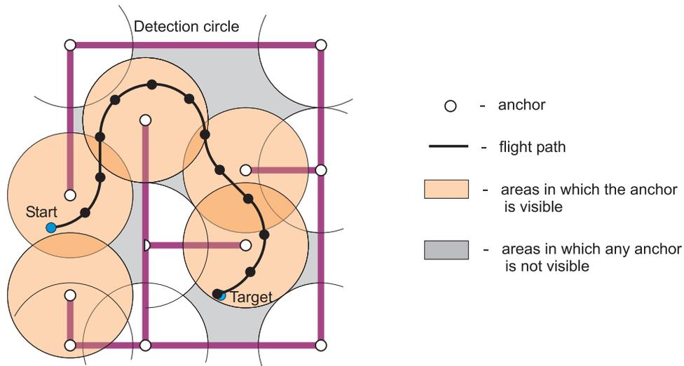
**Fig. 4. Indoor flight path with anchor-based planning.**
