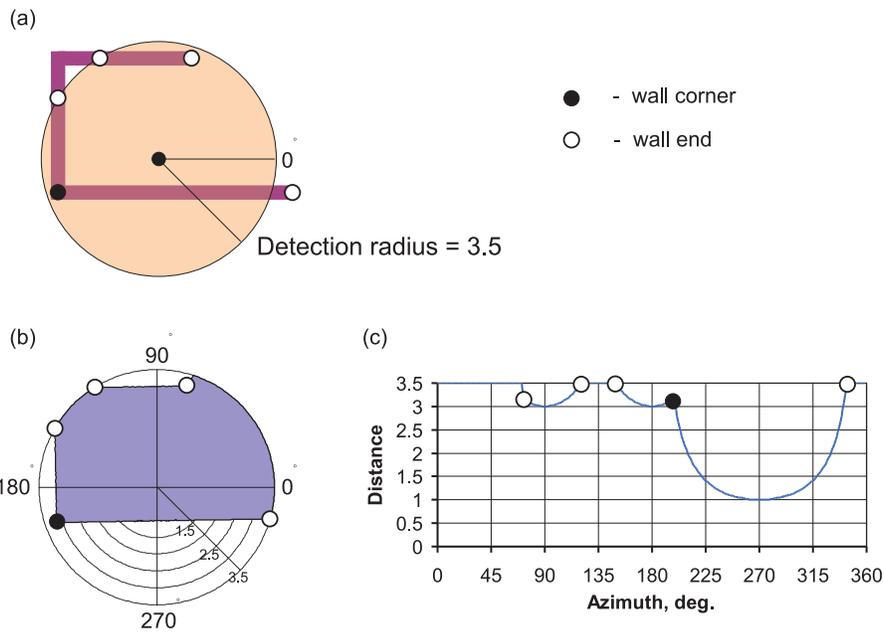
**Fig. 5. An example of anchor recognition by laser signal: (a) wall configuration; (b) azimuthal perspective; (c) signal versus azimuth angle.**
