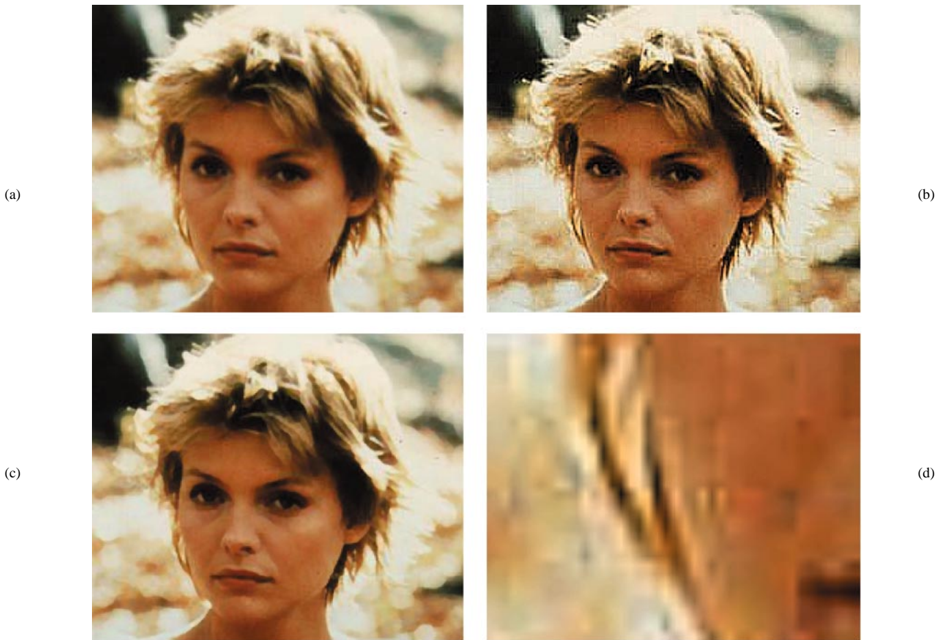
Fig. 9. Enhancement of a JPEG-compressed image. (a) Original image. (b) Unsharp masking applied to original image, after bilinear scaling \times 4 . (c) Enhancement and scaling \times 4 by proposed method. All images are shown at same size for presentation purposes only. Original image is compressed with quality 75%. The sharpening parameter used in the unsharp masking is 75%, a commonly used value. The graininess of the right image is due to the interaction of three components of the printer pipeline: Lossy JPEG compression, unsharp masking and printer halftoning. (d) Enlargement of selected area of (b) showing enhanced JPEG artifacts.
