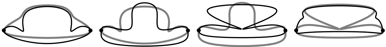
Figure 7: A Y -symmetric curve with a constant area has a positional constraint on the left and a tangential constraint on the right. Several direct manipulation operations are performed while, effectively, these two constraints keep the curve at a constant width , throughout. The previous operation is shown in gray and the new one is shown in black, from left to right. These examples were created in a few seconds.
