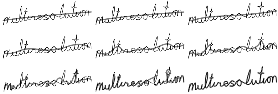
Fig. 2. Projections (in thick gray) of the original “multiresolution” curve from Figure 1 (in thin line) over different spline subspaces is presented. The top left is the smallest space (single quadratic polynomials) all the way to the bottom right which is the original space.
