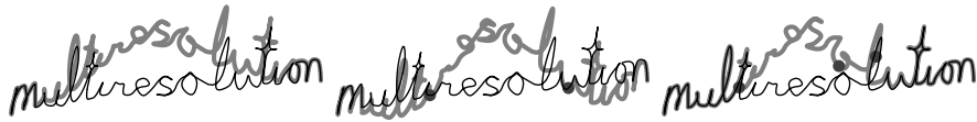
Fig. 4. Multiresolution editing without (a), and with two positional (b), and three tangential (c) linear constraints.
