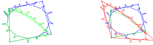
Fig. 7. Local area preserving multiresolution deformation. n = 7 , L = 2 . original curve (blue), deformed curve at level 2 (green), area preserving deformed curve at level 2 (red).
