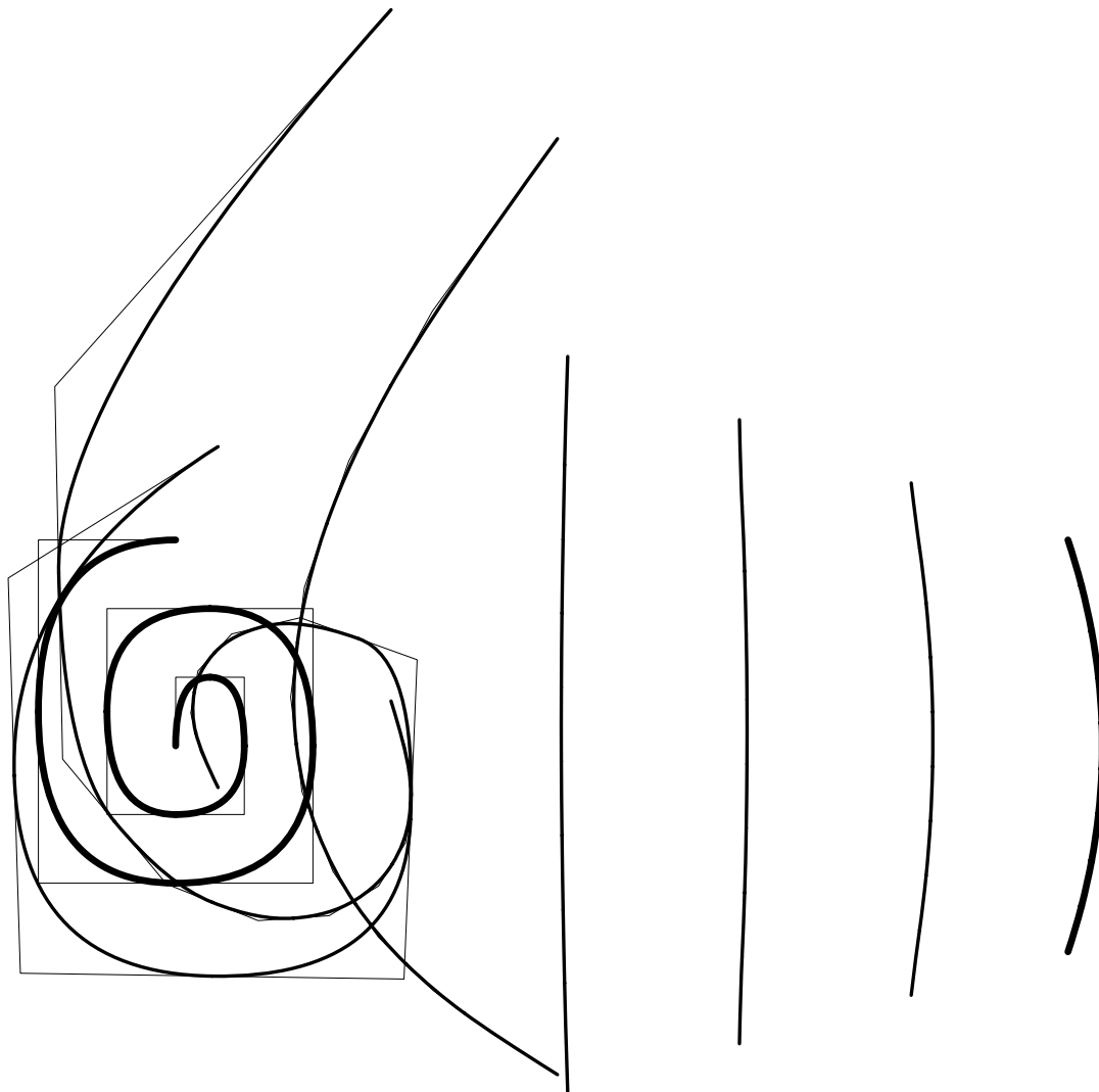
Figure 4: A metamorphosis of a B-spline curve to an almost straight curve using edge cutting, without self intersection. See also Figure 3.
