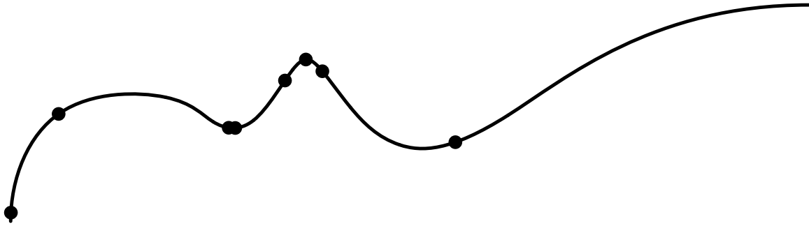
Figure 4: The points of extrema of \chi(t) = \kappa^2(t) computed as the zero set of \frac{d\chi(t)}{dt} . This includes both points of maximum curvature and points of minimum curvature, including inflection points.
