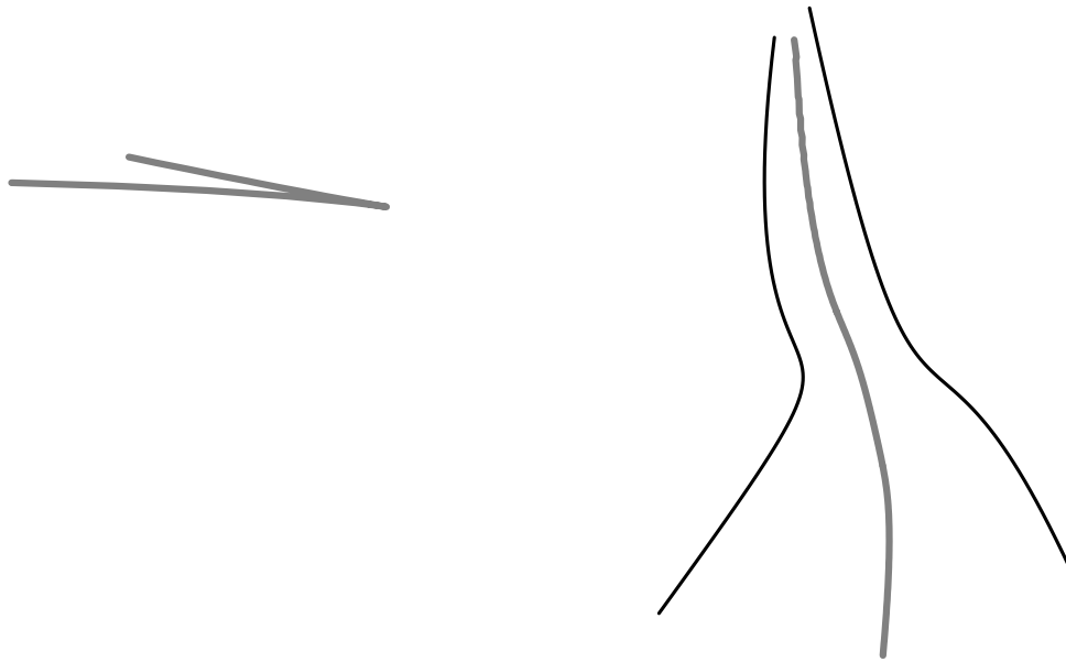
Figure 9: The bisector (bold curves) of two planar curves (light curves) can be approximated by computing the intersection of the plane containing the two curves with the bisector surface of the two curves rotated out of the plane by \epsilon degrees. In this example, we take \epsilon = \text{degree } 1^\circ .
