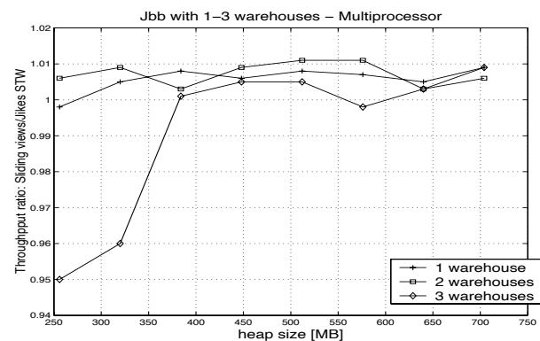
Figure 15: SPECjbb2000 on a multiprocessor: throughput ratio for 1-3 warehouses compared to the Jikes STW collector.
