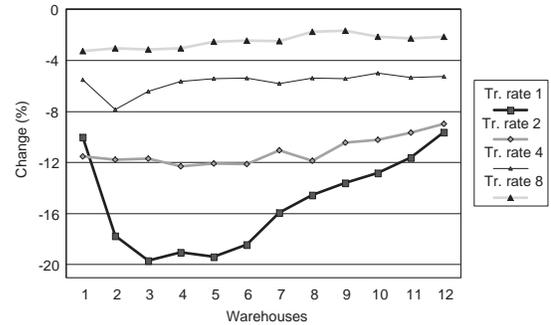
Figure 5: SPECjbb (AIX-6): Heap residency change between the base collector and the improved collector, for all tracing rates.
