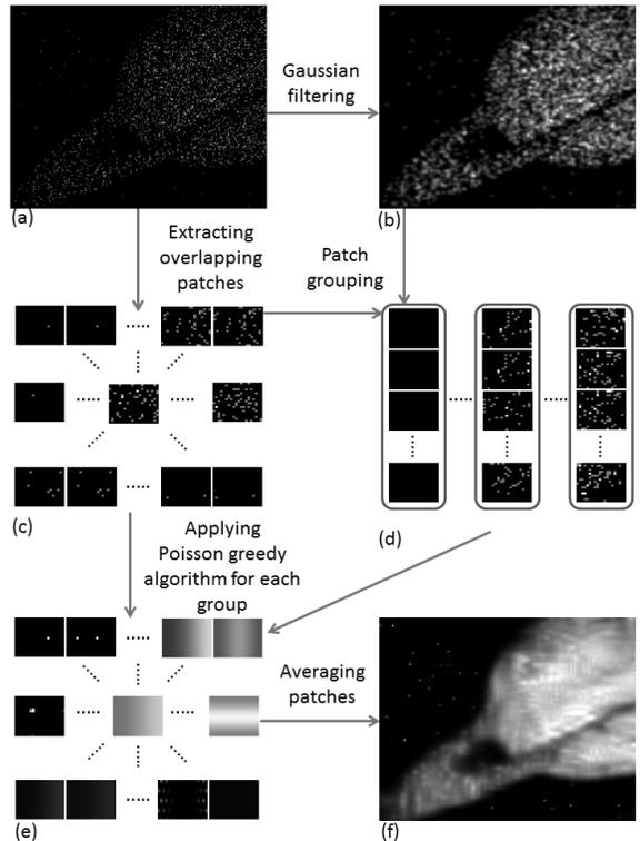
Fig. 2. The proposed model based Poisson denoising algorithm.
