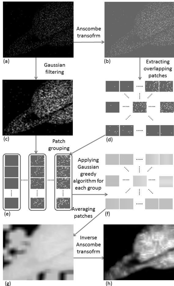
Fig. 1. The proposed Anscombe based Poisson denoising algorithm.
