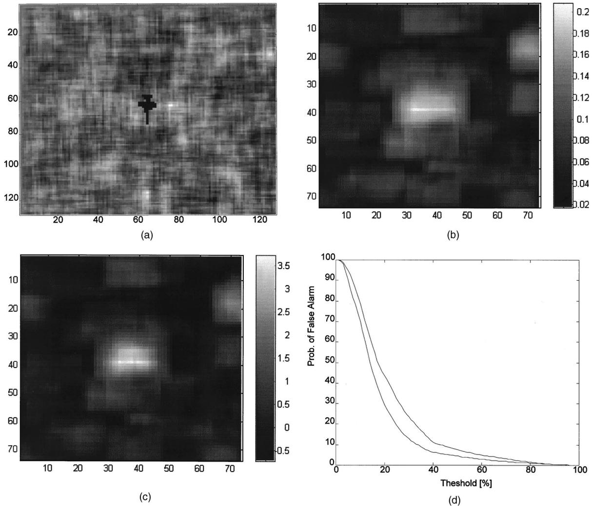
**Fig. 3** Results obtained for a stationary image with a Doyle-like statistical processing type: (a) input pattern, (b) output obtained after applying a conventional Doyle like processing, (c) output obtained after applying the contrasted approach, and (d) plot of the probability of false alarm as function of the applied threshold.
