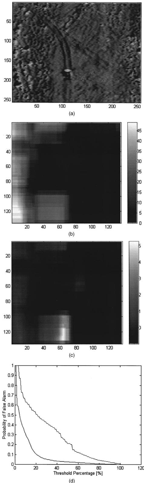
**Fig. 7** Results obtained for a real IR image with a POE statistical processing type: (a) input pattern, (b) output obtained after applying a conventional POE processing, (c) output obtained after applying the contrasted approach, and (d) plot of the probability of false alarm as function of the applied threshold.
