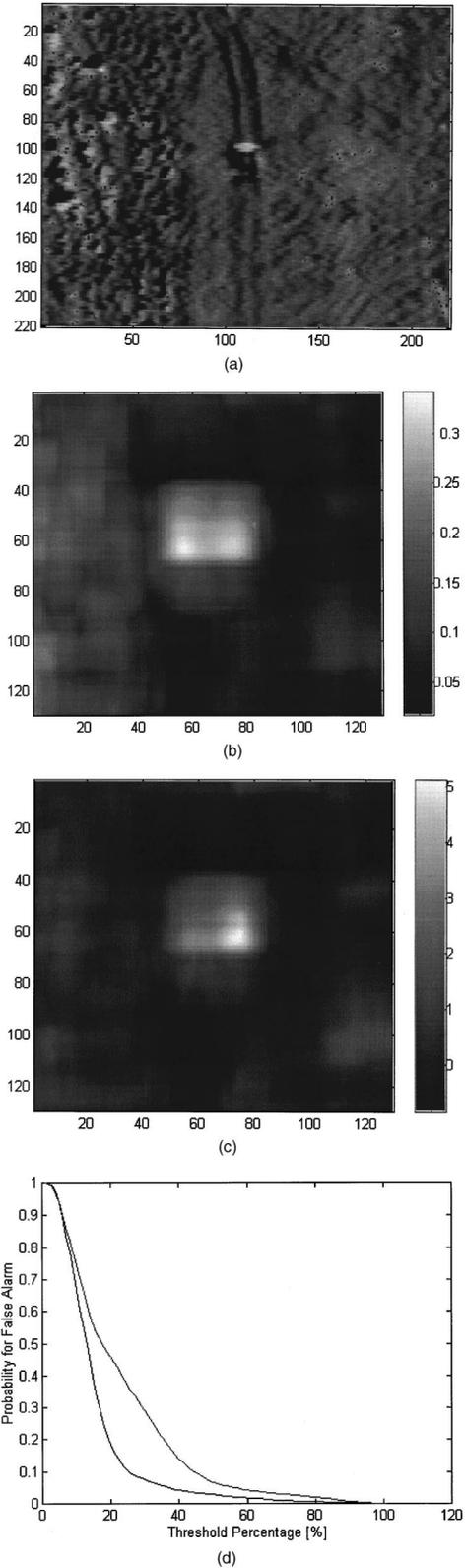
**Fig. 6** Results obtained for a real IR image with a Doyle-like statistical processing type: (a) input pattern, (b) output obtained after applying a conventional Doyle-like processing, (c) output obtained after applying the contrasted approach, and (d) plot of the probability of false alarm as function of the applied threshold.
