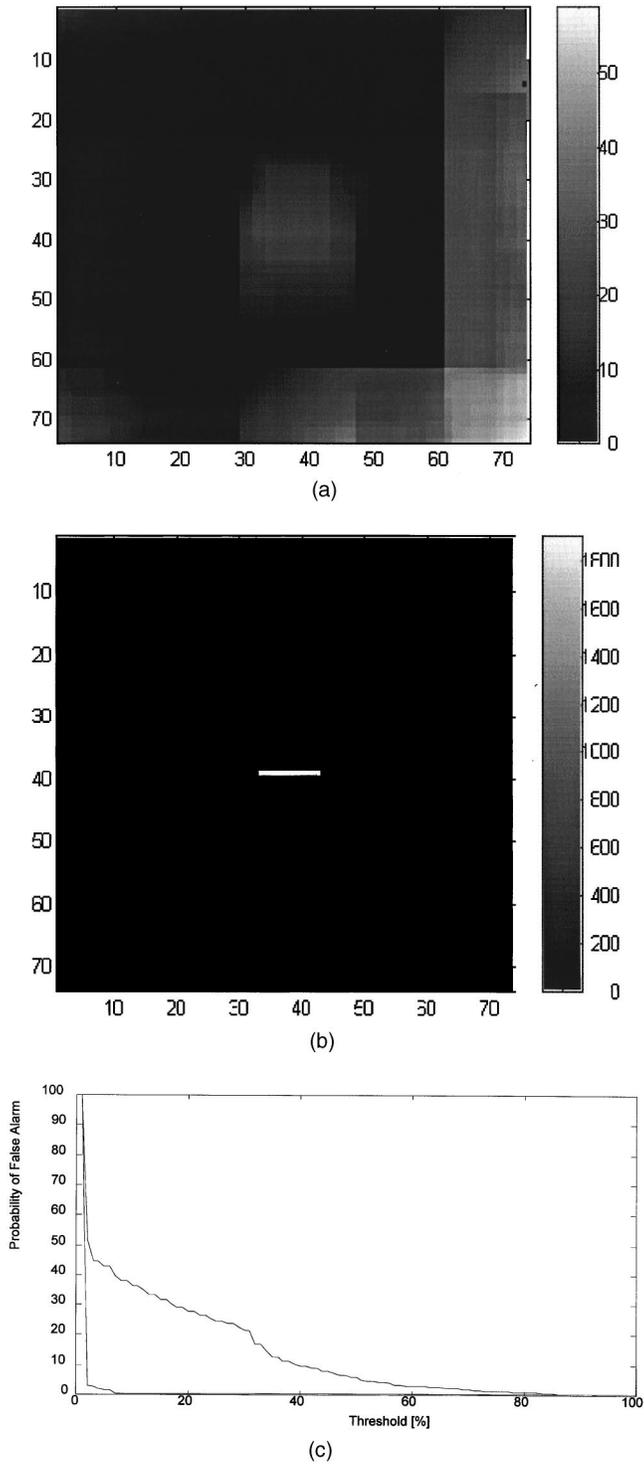
**Fig. 5** Results obtained for a nonstationary image with a POE statistical processing type: (a) output obtained after applying a conventional POE processing, (b) output obtained after applying the contrasted approach, and (c) plot of the probability of false alarm as function of the applied threshold.
