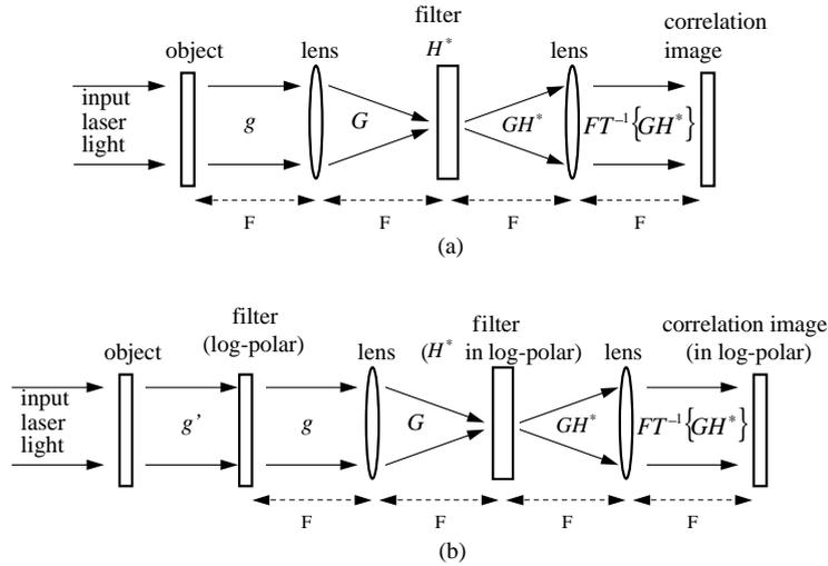
Fig. 1. The schematic implementation of the conventional correlators in optics: (a) The correlator based on the Fourier transform (used in detecting translations). (b) The correlator based on the Mellin transform (used in detecting rotation and scaling).  $FT$  denotes the Fourier transform,  $G$  and  $H$  are the Fourier transforms of the tested image and the reference image accordingly, and  $F$  is the focal length of the lenses.
