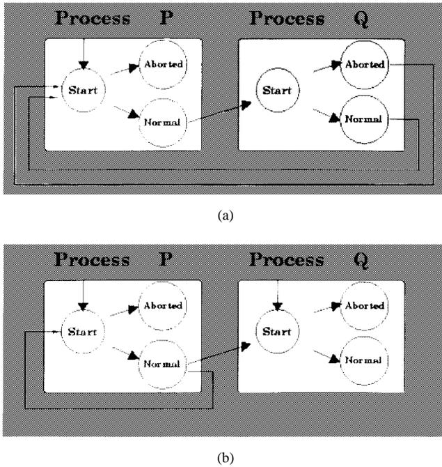
Fig. 1. (a) Synchronous recurrent composition; (b) asynchronous recurrent composition.
