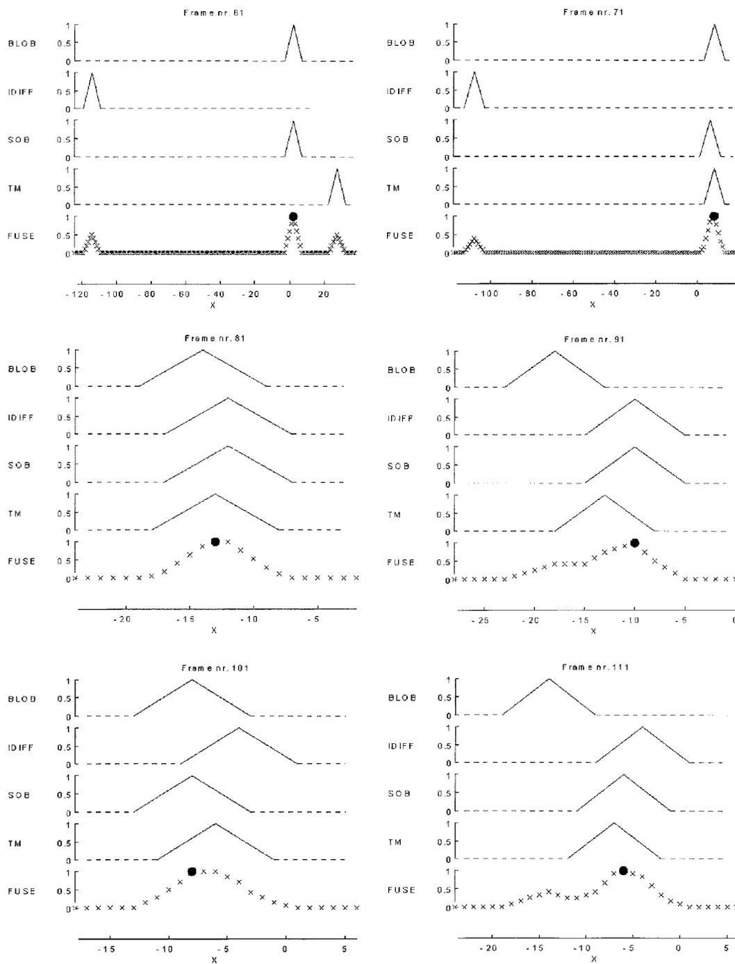
Fig. 7. (Continued.) Sequence showing the tracking results and the fusion process. During the sequence, the camera is driven by the fusion module. The plots present each module's votes for each action (here motion in the horizontal direction). These votes are combined by the fusion module (FUSE), and the best action indicated by the dot in the plots is selected. Sequence showing the tracking results and the fusion process.
