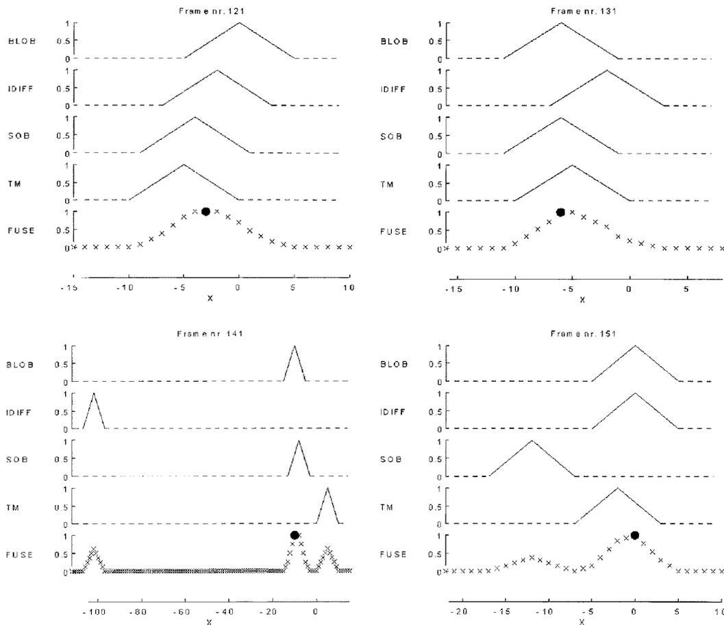
Fig. 7. (Continued.) Sequence showing the tracking results and the fusion process. During the sequence, the camera is driven by the fusion module. The plots present each module's votes for each action (here motion in the horizontal direction). These votes are combined by the fusion module (FUSE), and the best action indicated by the dot in the plots is selected. Sequence showing the tracking results and the fusion process.
