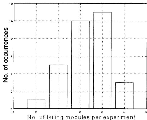
Fig. 4. Distribution of the number of failing modules at each trial during 30 trials. The fusion module is not taken into consideration here. Setting complexity increases from left to right.
