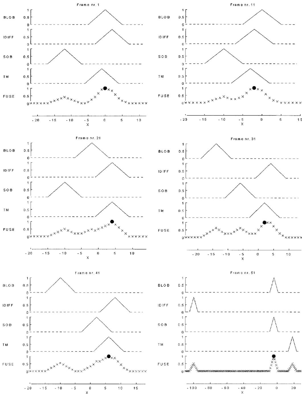
Fig. 7. Sequence showing the tracking results and the fusion process. During the sequence, the camera is driven by the fusion module. The plots present each module's votes for each action (here motion in the horizontal direction). These votes are combined by the fusion module (FUSE), and the best action indicated by the dot in the plots is selected. Sequence showing the tracking results and the fusion process.
