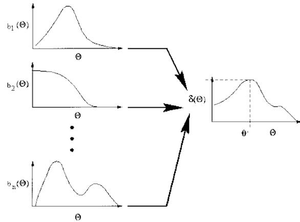
Fig. 2. Schematic of the composition process in a team of homogeneous modules. The modules generate their votes (left), which are combined using the composition operator. The composed module is illustrated on the right.
