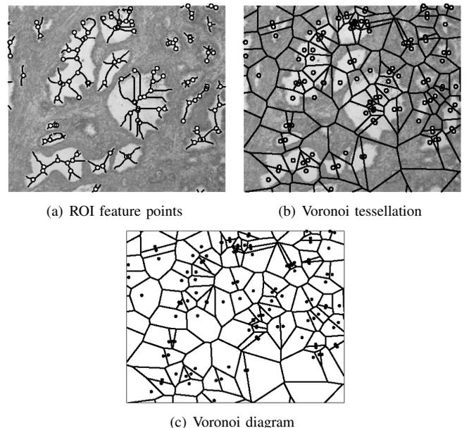
Fig. 5. The process of constructing the Voronoi tessellation of the ROI for verification acceleration. The junction points of glands object skeletons are marked by white dots in (a).
