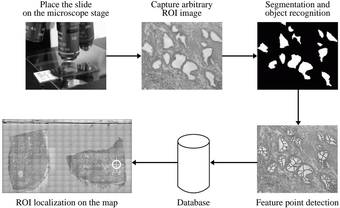
Fig. 4. Outline of the algorithm localization stage. The ROI image is segmented and the typical objects are identified. Then the feature points are extracted from the objects and ROI localization followed by position verification is performed.
