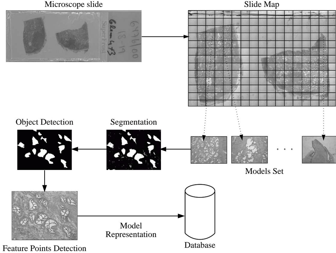
Fig. 3. Outline of the algorithm preprocessing stage. First, the slide map is constructed from small adjacent images captured by a microscope imaging system. Then the slide map is divided into parts corresponding to a model set. After that the feature points of each model are identified. Finally, the model representation is calculated and stored in the database.
