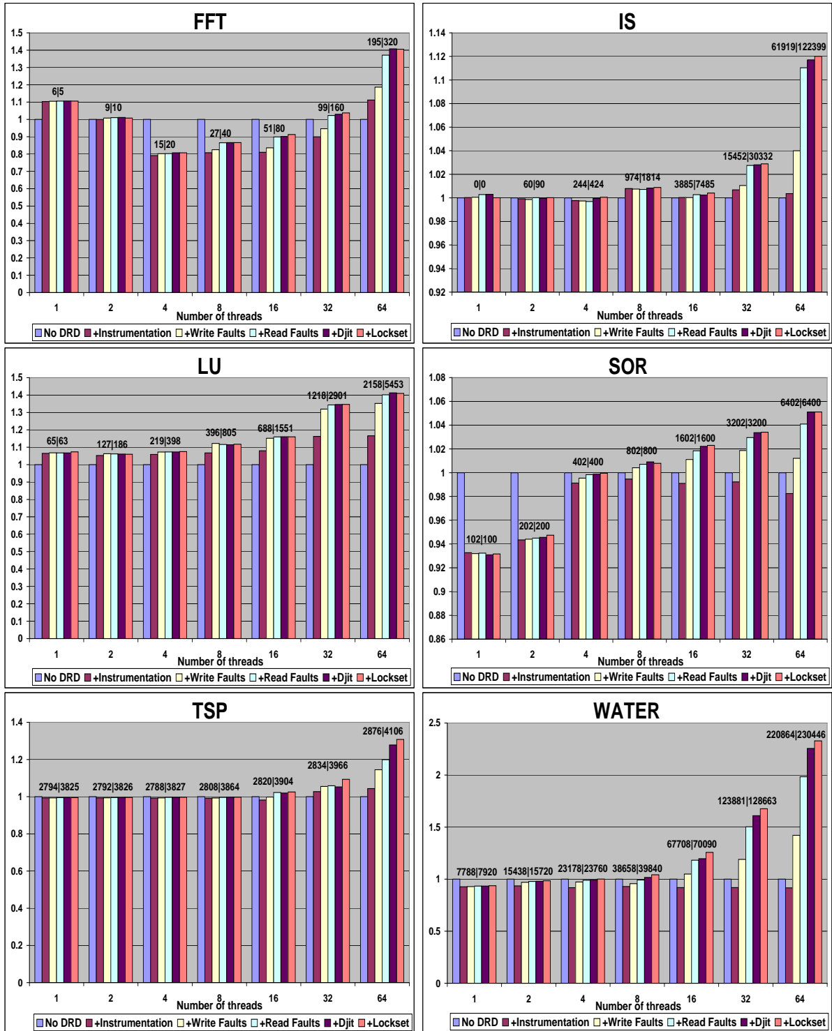
Figure 19: Breakdowns of the overheads measured for the benchmark applications. The times are relative to the original uninstrumented version with the corresponding number of threads. The numbers above the bars indicate, respectively, the number of write and read faults.
