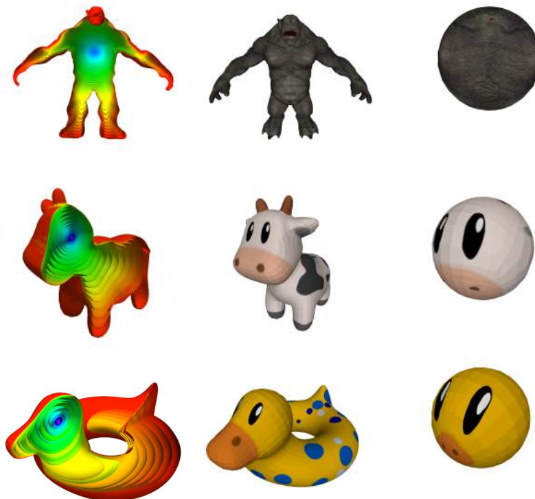
Figure 5.10: Applying texture. (left) The result of our flow. (middle) Initial mesh textured. (right) Final mesh textured, zoomed in.
