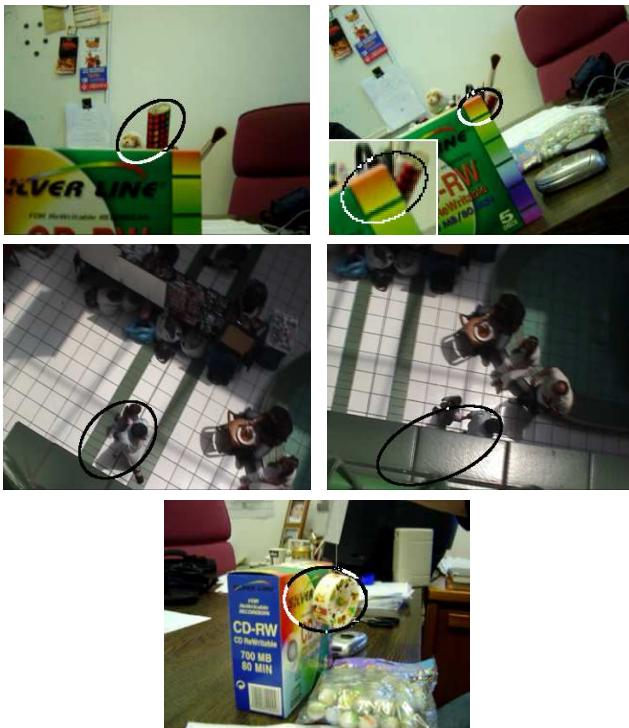
Figure 11: Results obtained using the proposed tracker without its boundary-related kernel ( \alpha = 0 ). It is evident that color edges play a crucial role in the proposed tracker.
