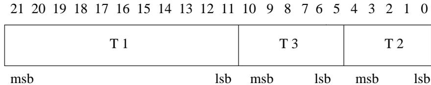
Fig. 5. The coding of COUNT
