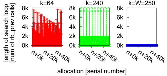
Figure 9: *Length of the `alloc_iova` search loop under the EIOVAR<sub>k</sub> deferred protection regime for three  $k$  values when running Netperf TCP Stream. Bigger capacity implies that the searches become shorter on average. Big enough capacity ( $k \geq W = 250$ ) eliminates the searches altogether.*
