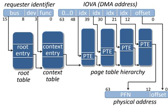
Figure 1: IOVA translation using the Intel IOMMU.
