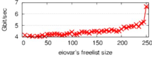
Figure 8: *Under deferred protection, EIOVAR<sub>k</sub> eliminates costly linear searches when k exceeds the high-water mark W.*
