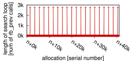
Figure 3: The length of each alloc\_iova search loop in a 40K (sub)sequence of alloc\_iova calls performed by one Netperf run. One Rx-Tx interference leads to regular linearity.
