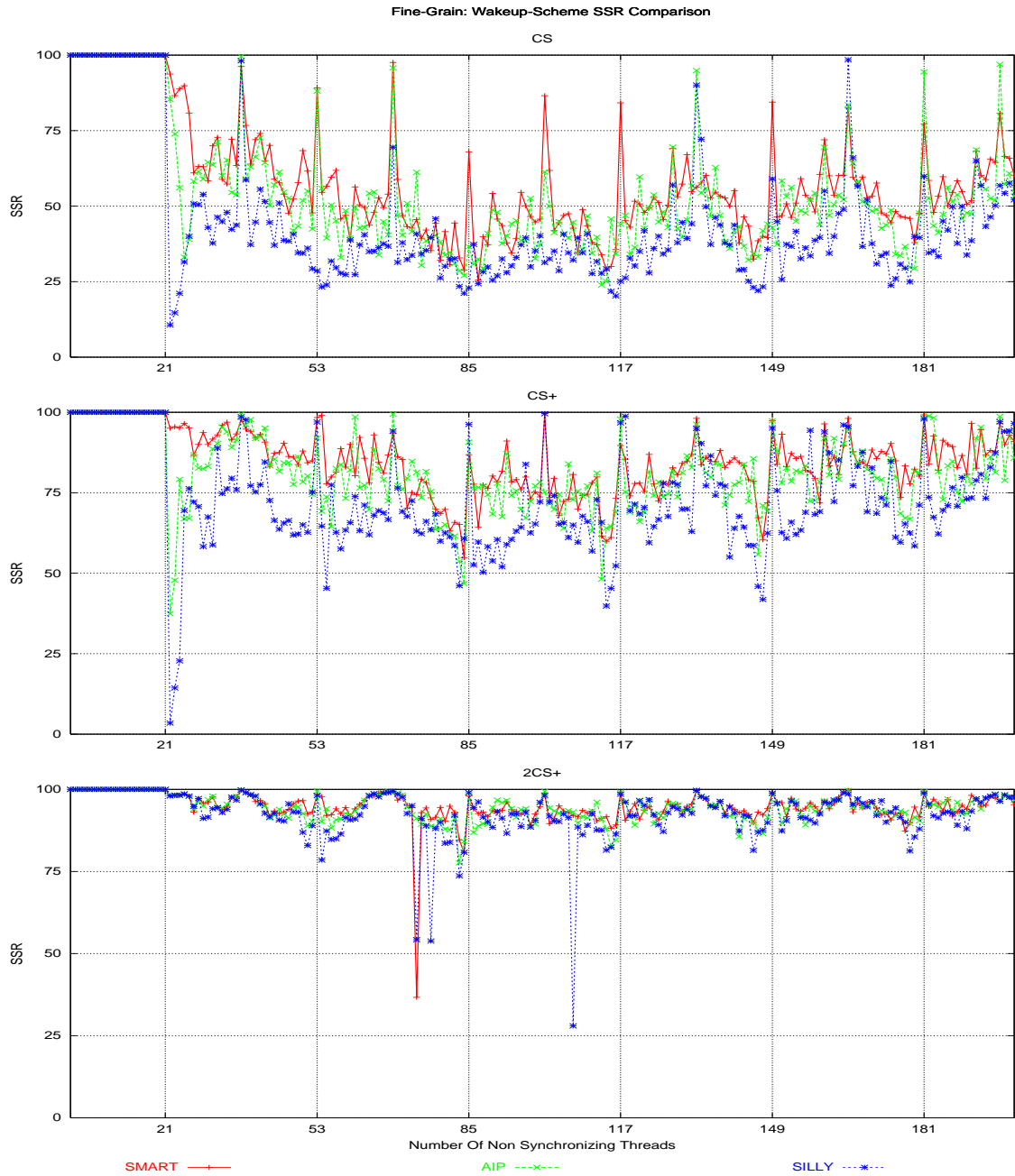
Figure 7.7: This figure compares the SSR achieved by fine grain jobs when different wakeup schemes and maximal spin durations are used. Generally, bigger spin duration resulted in better SSR. For 2CS+ most measurements are in 80-100% ( avg \approx 96\% ), for CS+ in 50-100% ( avg \approx 77\% ) and for CS in 25-75% ( avg \approx 47\% ). This means that when choosing a correct spin duration, a fine grain synchronizing job within a non-synchronizing environment may successfully compute regardless of the load. When examining the difference between the various wakeup schemes, we see that the difference is fairly small, and shrinks as we enlarge the spin duration (in 2CS+ the the curves are almost indistinguishable).
